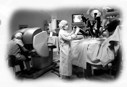
The Da Vinci robotic arm allows surgeons to operate through small incisions. It also makes operating at a distance possible.
