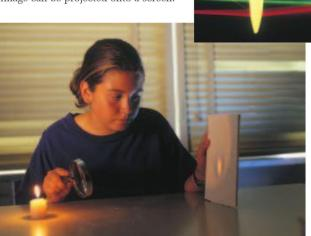
Figure 2.27 Convex lenses bring light rays together.
