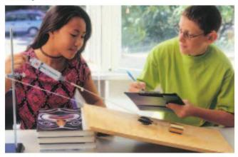
Figure 2.8 The measured mechanical advantage of this system was less than the speed ratio when the students tested it.
