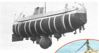
Figure 4.11 The bathyscaph Trieste made it to the bottom of the Marianas Trench in 1960. A bathyscaph consists of a large float with a metal sphere underneath. The sphere is where the people sit.
