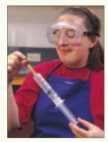
**Figure 3.14** Step 1. The plunger should be three-quarters of the way up the tube.
