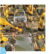
Figure 3.17 Assembly-line robots weld car bodies together in an automobile factory.
