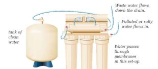
**Figure 1.10** This reverse osmosis set-up can also create pure water from salty or polluted water.
