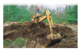
Figure 2.14 The fluid in the hydraulic system of this backhoe transmits forces that move the levers for lifting heavy loads.
