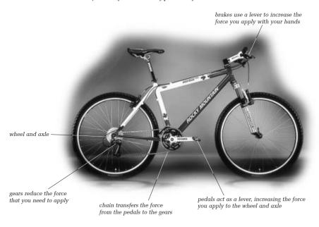
**Figure 1.22** A bicycle is a complex machine made up of simple machines that work together. The whole bicycle is a system, made up of many subsystems.
