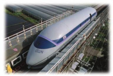
**Figure 3.15** Because they float on magnets, MAGLEV trains experience very little friction. This enables them to use more of their energy for increasing speed rather than opposing friction.
