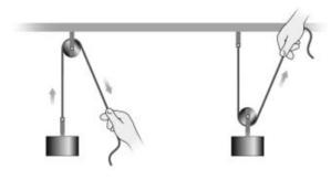
$\textbf{Figure 1.10} \ \ \text{Two types of pulleys}$
