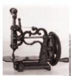
**Figure 3.14a)** Early sewing machines were operated by a hand crank. They could sew only simple stitches.
