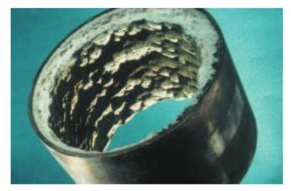
**Figure 1.4** Hard water causes mineral deposits called *scale* to form on the inside of pipes. The scale clogs up the pipes.
