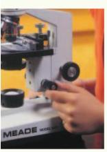
Figure 2.8 Using the fine adjustment knob
