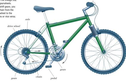
Figure 1.25 In a bicycle, the chain is the linkage that drives the gearwheels. When you shift gears, you move the chain from the larger gearwheel to the smaller ones or vice versa.
